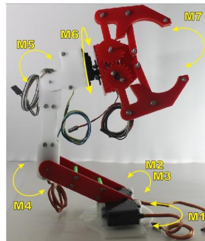
Figure 6. Servo motor movement on the robotic arm
