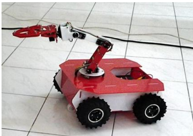
Figure 1. Robot Transporter with the robotic arm
